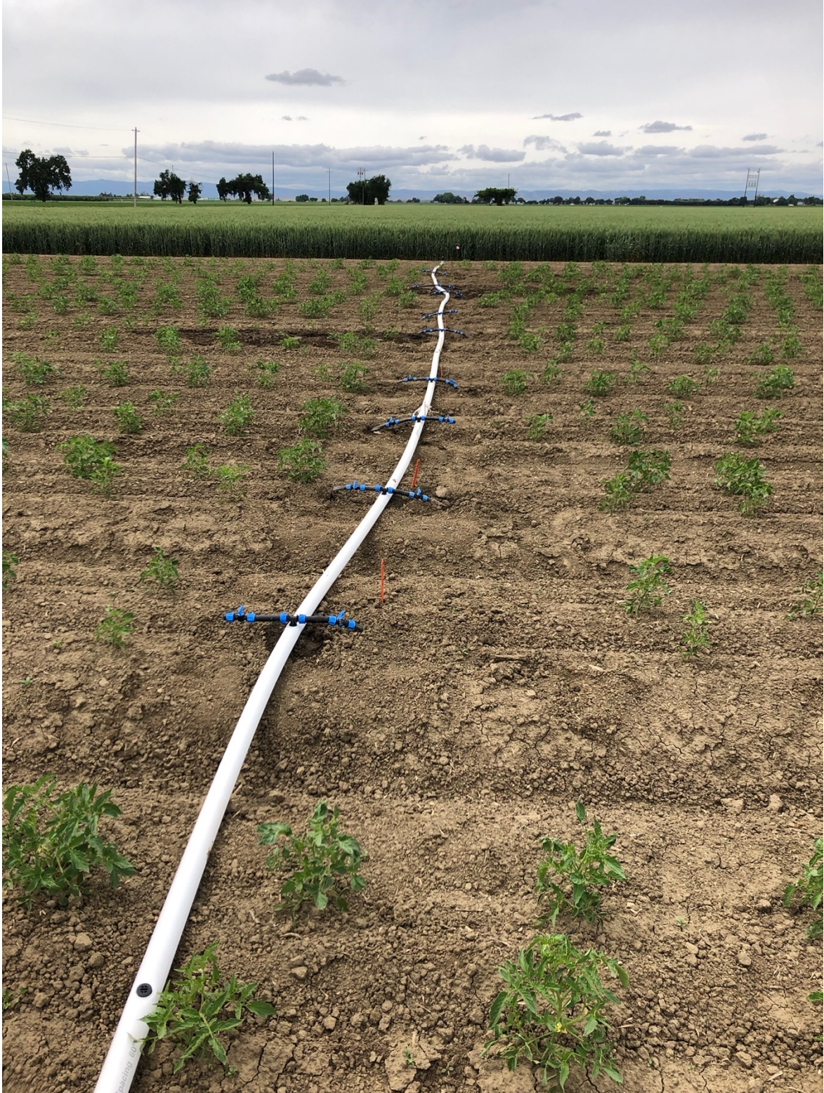
Figure 2. Valved connections at each plot allowed two replicates to be treated at once. A valve was located at the end of the layflat line to flush line in between treatments.
