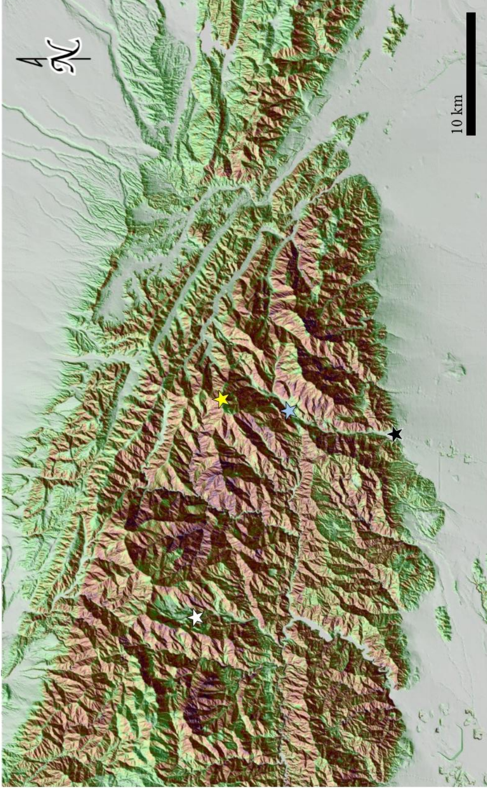
Figure 4: The San Gabriel Mountains are an area of high elevation and steep slopes. This image shows slope overlain on a hillshade image from Cal-Topo (green: low slopes, red: steep slopes). The stars indicate the following locations: White— Crystal Lake rock avalanche deposit, Yellow— Mt. San Antonio Peak, Blue— Mt. Baldy Village, Black— San Antonio Dam.
