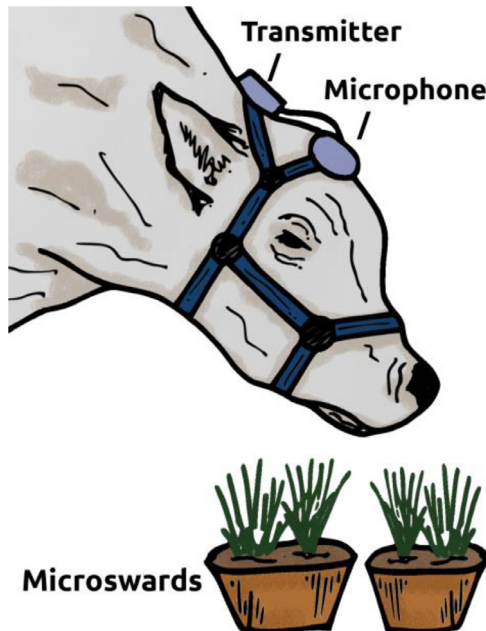
Fig. 2. Microphone was located facing inwards on the forehead of the cow and the transmitter was placed on the neck. The cow is grazing microswards.
