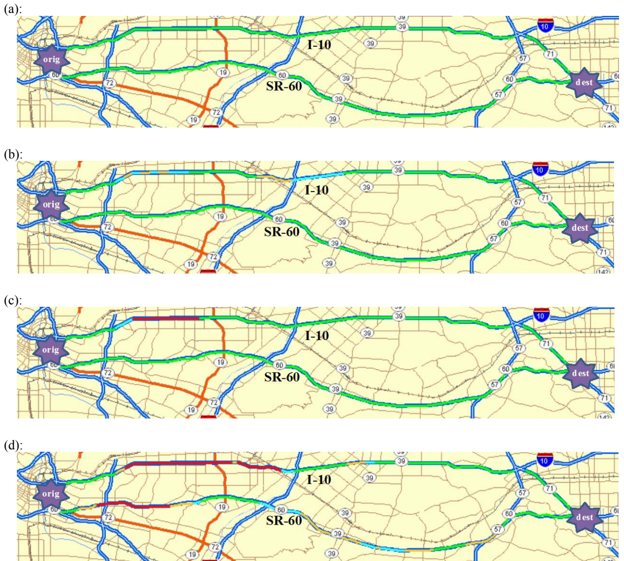
Figure 3.3: (a): Road network for case study 1: free-flow conditions on both freeways between Los Angeles and Chino; (b): Road network for case study 2: free-flow conditions on SR-60 and moderate congestion on I-10; (c): Road network for case study 3: mostly free-flow conditions on SR-60 and heavy congestion on I-10; (d): Road network for case study 4: moderate condition on SR-60 and heavy congestion on I-10. Note that roadway links are colored based on their real-time speeds( 0-40 km/h” magenta; 40-65 km/h: orange; 65-90 km/h: blue; 90+ km/h: green). This also applies to (b), (c), and (c).
