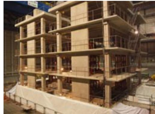
Figure 5-2. Overview of test set up on the shaking table
