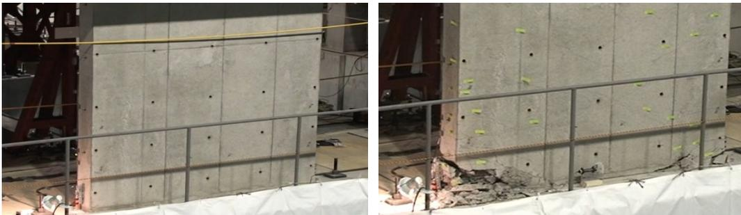
Figure 5-16. Damage on the RC shear walls (Axis A) at (a) 50%, (b) 100% Kobe record
