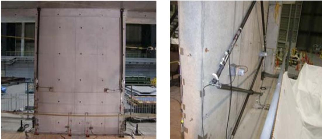
Figure 5-9. Instrumentation of the RC shear walls
