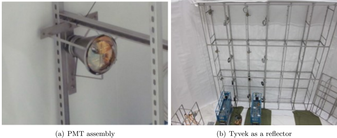
Figure 5-3: 8-inch PMTs and Tyvek film in the water pool of the Daya Bay experiment.
