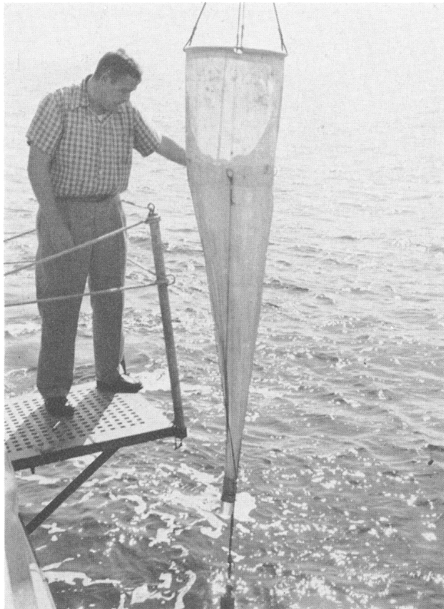
FIGURE 4. Plankton net used in collecting food organisms of sardine. Photograph by Kramer Adams, October, 1949.
