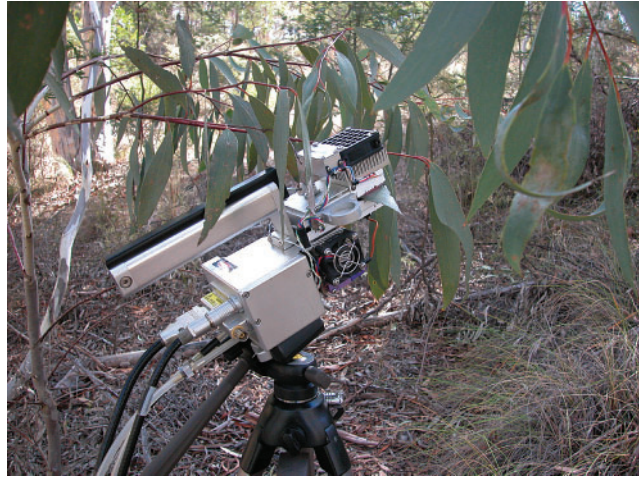
Fig. 1. Measuring leaf gas exchange in Eucalyptus pauciflora using a LI-6400. Photography by M. Harrison.
