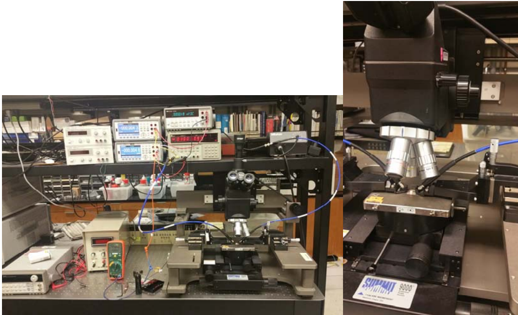
Fig. 6.11: Pictures of the DC Measurement Bench.
