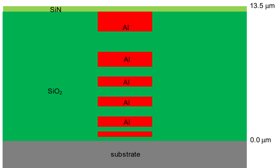
Fig. 3.2: HBT Example Process Cross Section.
