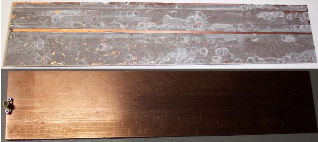
Fig. 1.6: Top (top figure) and Bottom (bottom figure) of Microstrip Line.
