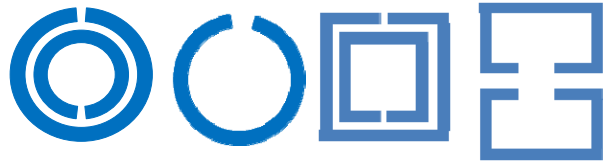
Fig. 2.1: Negative Permeability SNG Metamaterials.
