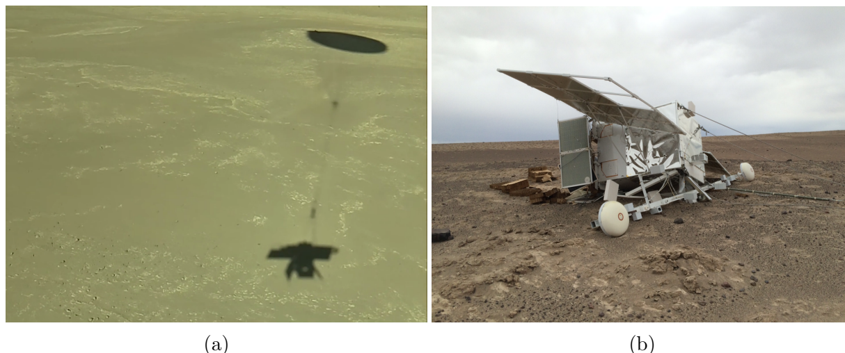
Figure 3.2: Left: A still from a video shot from the gondola, moments before landing in the Atacama desert. The shadow of the COSI payload and parachute are clearly seen on the desert floor. Right: A photograph taken by the recovery team of COSI at its landing site. The exterior structure sustained damage, but the instrument and electronics were recovered in excellent shape.
