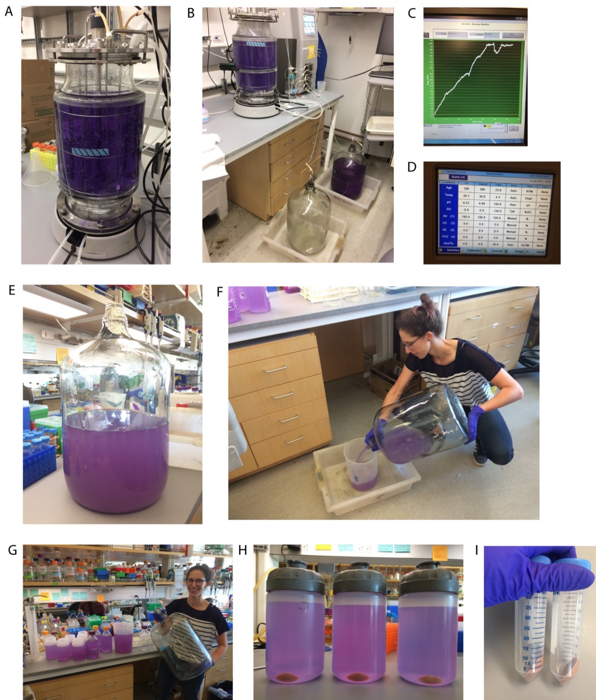
Figure S14. Growing 20L of H. neapolitanus in a chemostat. (A) The chemostat setup. (B) Chemostat setup showing the input and output media collection bottles. (C) Continuous optical density (OD) graph. (D) Summary page of the control software. (E) Cells ready for harvesting. (F) Squat, don't bend your back, when lifting heavy things! (G) Pretty purple culture that is ready to spin down. (H) Agonizingly small pellets for each 1L bottle. (I) Tubes of 3g of cell pellets from 7L each that are ready for freezing at -20^{\circ}\text{C} .
