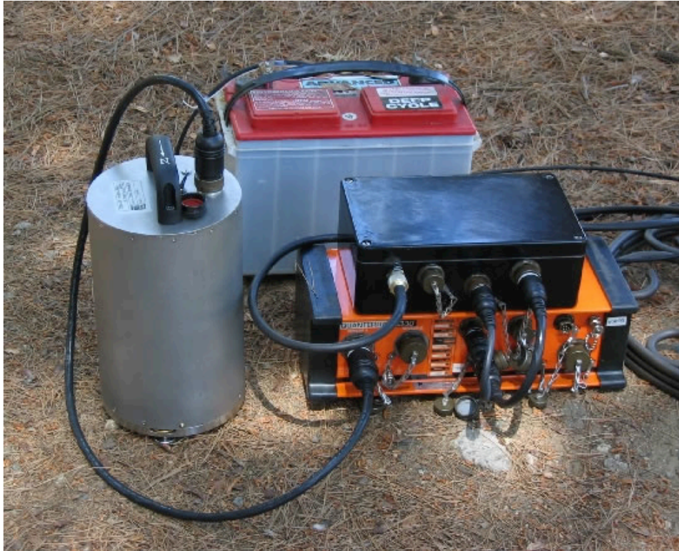
Figure 2.2: The set of instruments for one node of a wireless network: a seismic sensor, CDCC, digitizer (Kinometrics Q330), and car battery.
