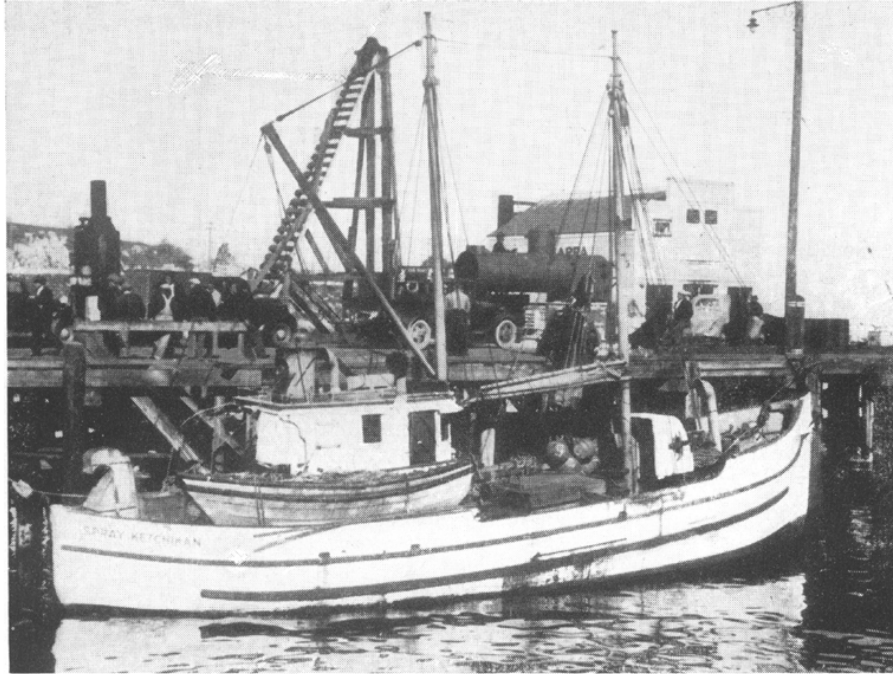
Figure 3. Northern halibut boat. Note the chute on the stern for paying out set line. Photograph by Robert D. Byers
