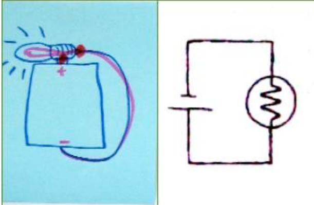
Figure 5.6. Iconic (left) and schematic (right) drawings of complete circuits with lit bulbs.
