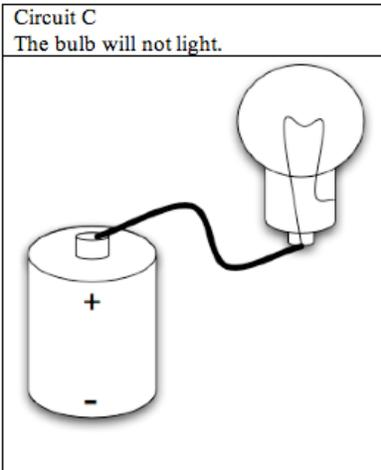
Figure 3.2. Diagram of an incomplete circuit.
