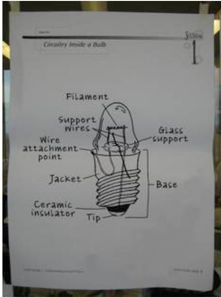
Figure 5.4. Close-up image of the “architecture of the light bulb” wall chart.
