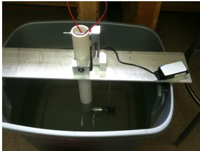
Figure 5.12: Motor force test platform: submerged motor unit is attached to an extended arm which pivots against a force transducer. Power is applied to the motor at a range of values, and output force is recorded in Matlab.
