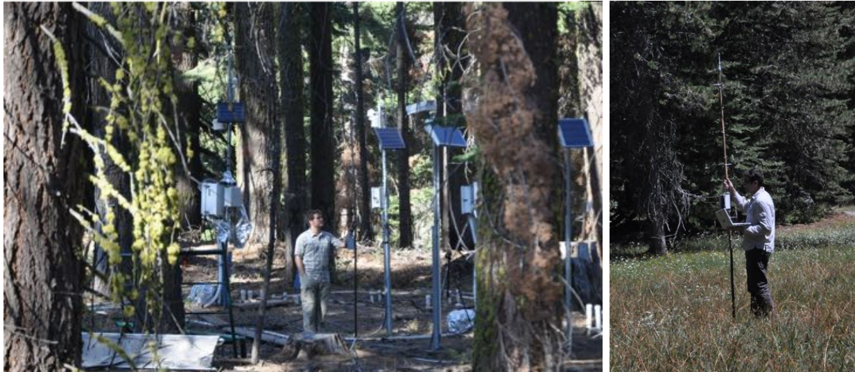
Figure 3.1: Packet delivery ratio was measured using L-COM HGV-2404U 4dBi antennas at representative locations near the existing network.
