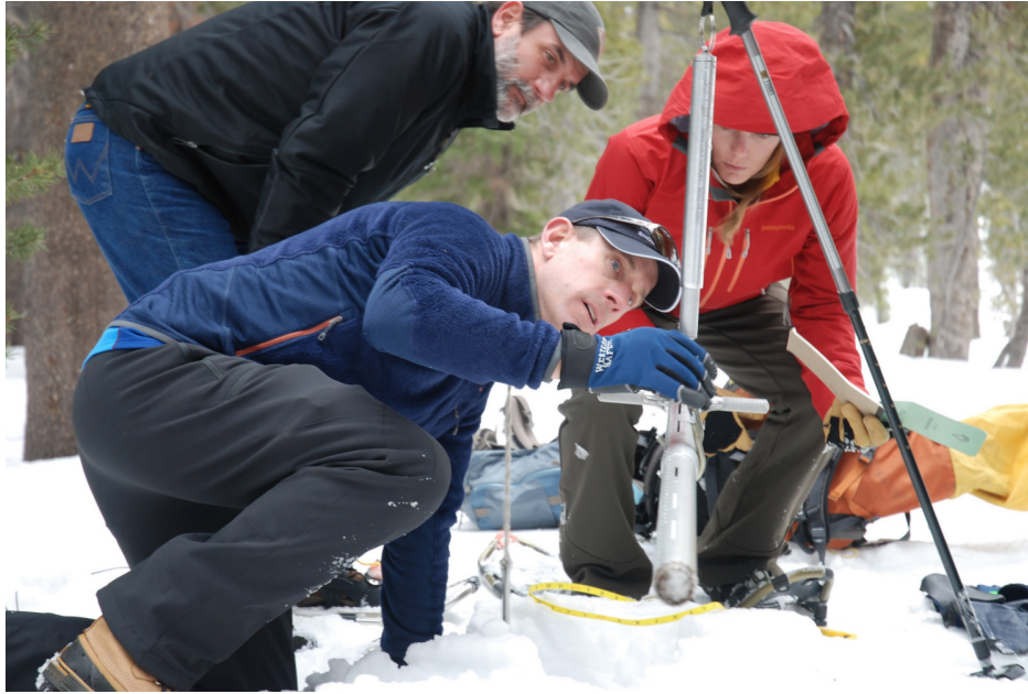
Figure 1.1: Conducting a synoptic snow survey. Measurements are taken by personnel at representative regions across the landscape.
