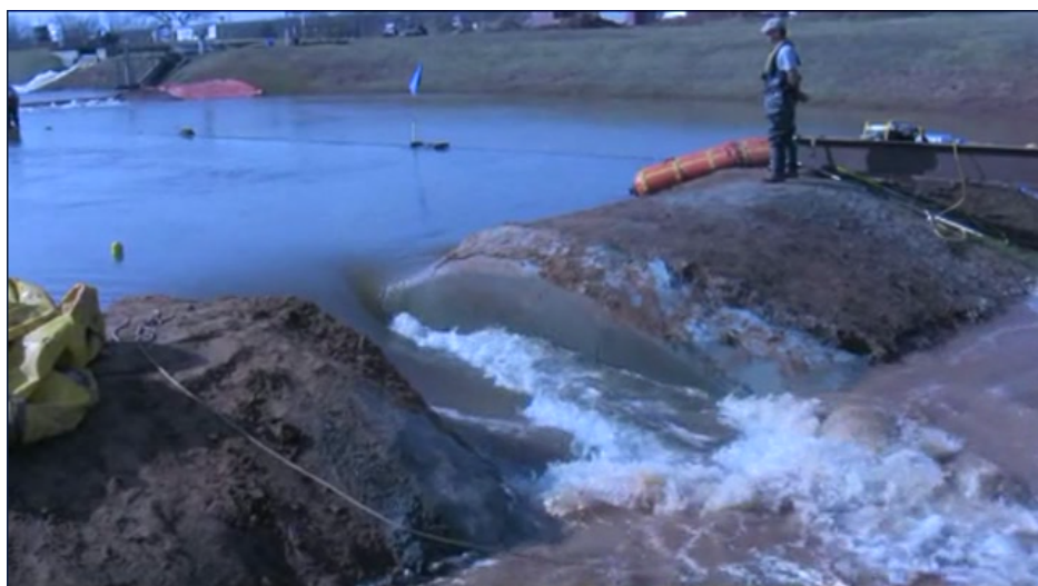
Figure 5.29: Floating sensor about to pass through the breach.
