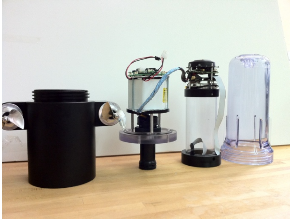
Figure 5.7: Modular structure of vehicle's internals: (from left to right) Delrin lower hull with removable motor pods, lower electronics assembly with battery and sensors, upper electronics assembly with microprocessors and guidance/location sensors, and clear PVC upper hull.
