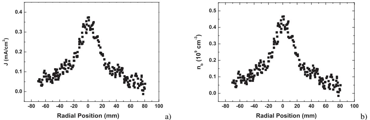
**Fig. 3** The reference supersonic ion beam density: a) current density,  $J$  ( $\text{mA}/\text{cm}^2$ ) and b) number density,  $n_b$  ( $\times 10^9 \text{ cm}^{-3}$ ) at 80 watt RF power input with  $f = 18.75 \text{ MHz}$  and  $3 \times 10^{-4} \text{ Torr}$ .
