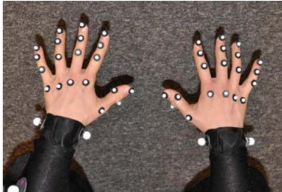
Figure 2.4: Hands outfitted with a fairly comprehensive marker set for optical motion capture. Further markers could be added to capture the motion of additional joints such as the CMC joint.
