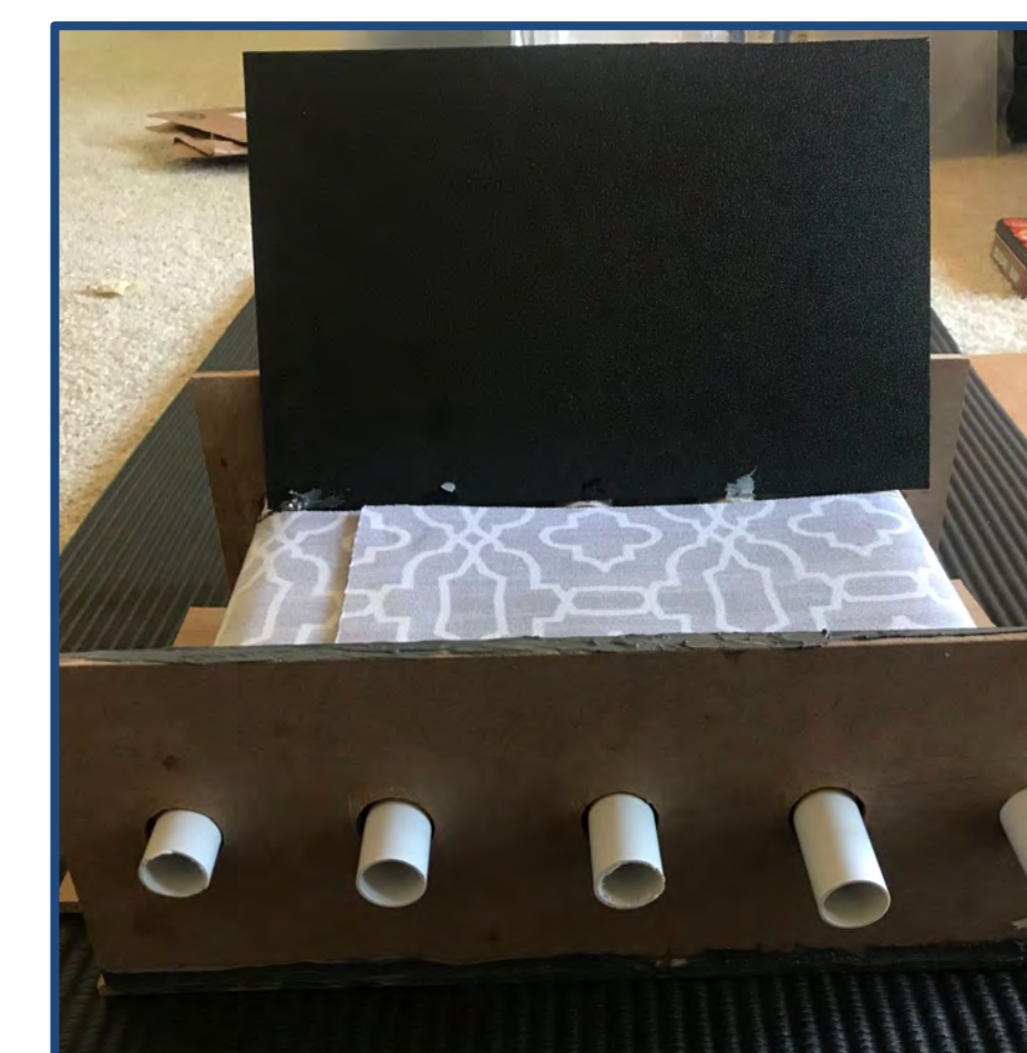
Figure 8: Conveyor Belt Structure
