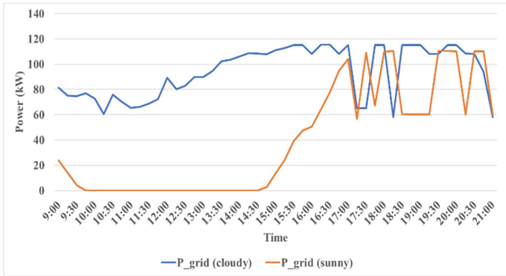
Figure 3.24 Cloudy Day & Level II Activity: Power Purchased from Grid
