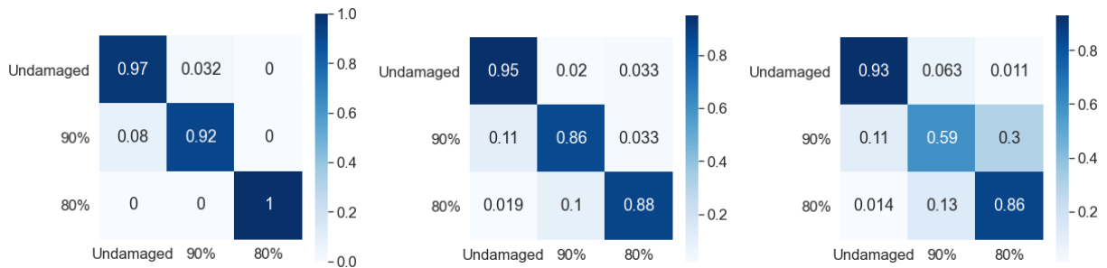
Figure 5.2: Confusion matrices of Task 3 for the model with \# of units = 50 for the RC frame: floor 1 (left), floor 2 (middle), and floor 3 (right).
