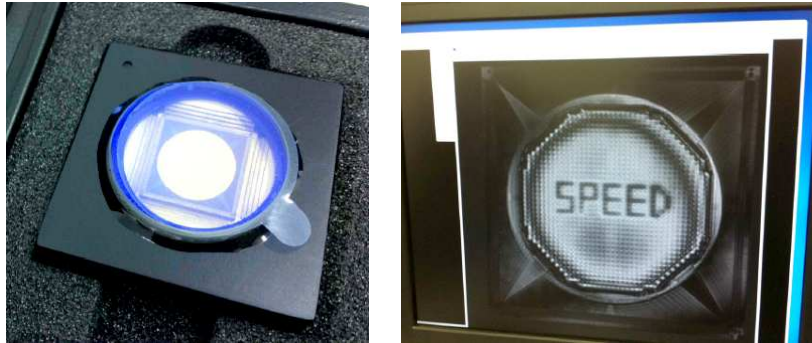
Figure 7. Left: picture of one of the two deformable mirrors (Kilo-C-DM) from Boston Micromachines manufacturer, Right: picture of a DM taken by a ZYGO interferometer with activation of some actuators.
