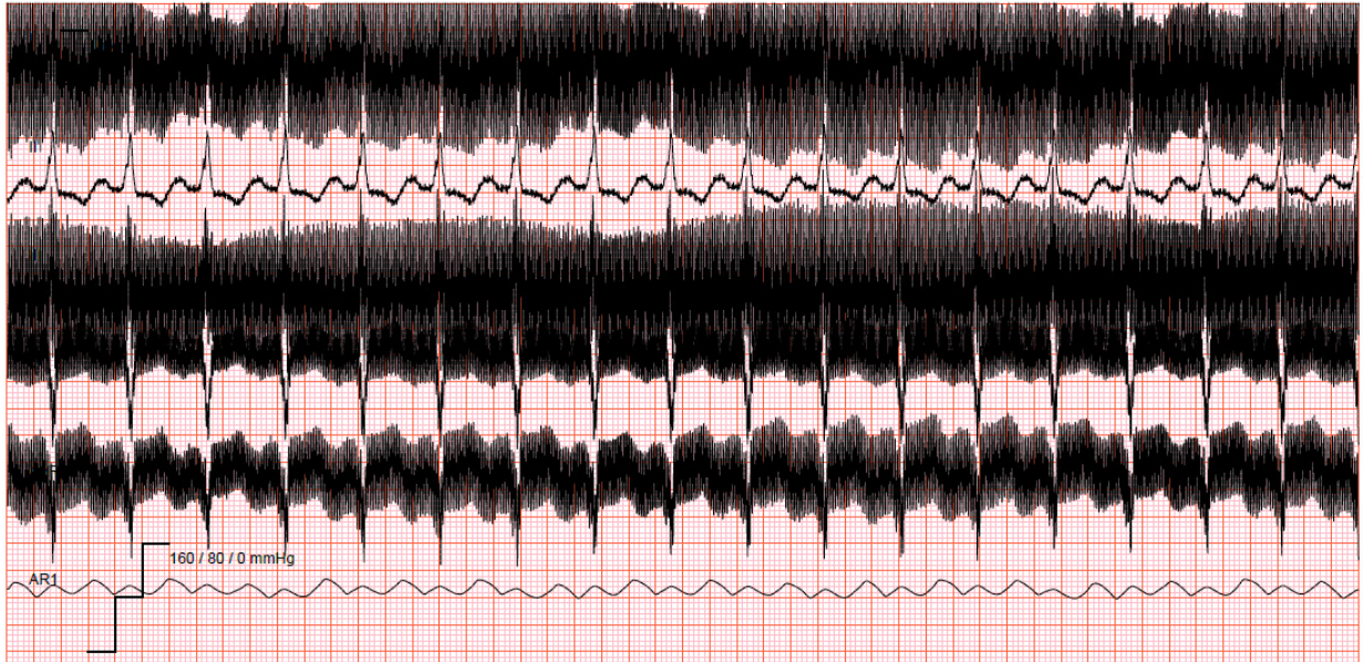
Figure 2. Example of 60-cycle interference on an electrocardiogram (ECG) obtained from the bedside monitor in a patient with a left ventricular assist device. Note the clean ECG signal in lead II, heart rate 105 beats/minute, and non-pulsatile arterial blood pressure waveform (bottom). The arterial blood pressure is 100/84 and the non-invasive blood pressure is 102/62.
