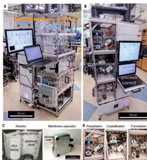
Figure 4.1 A reconfigurable system for continuous production and reformulation of APIs. [Source: ref 25]
