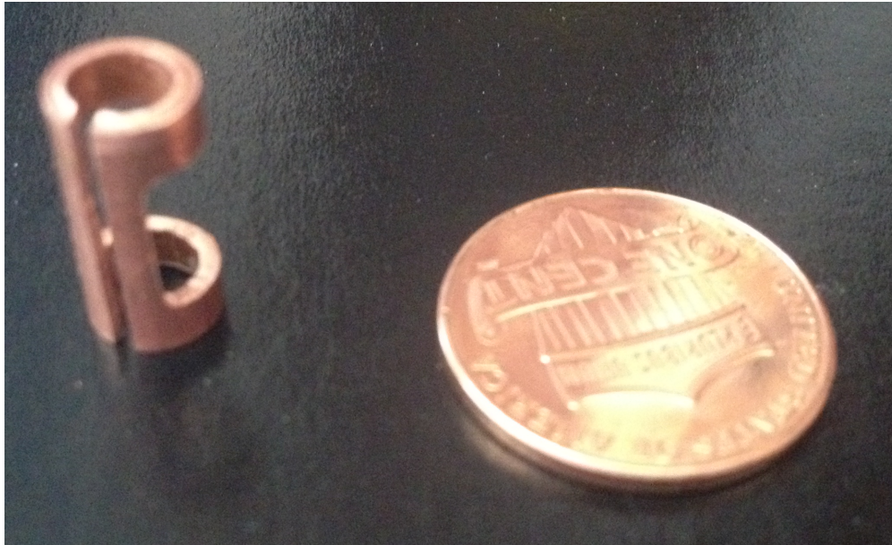
Figure 2.5: The blank for the MAG resonator with a penny for scale.
