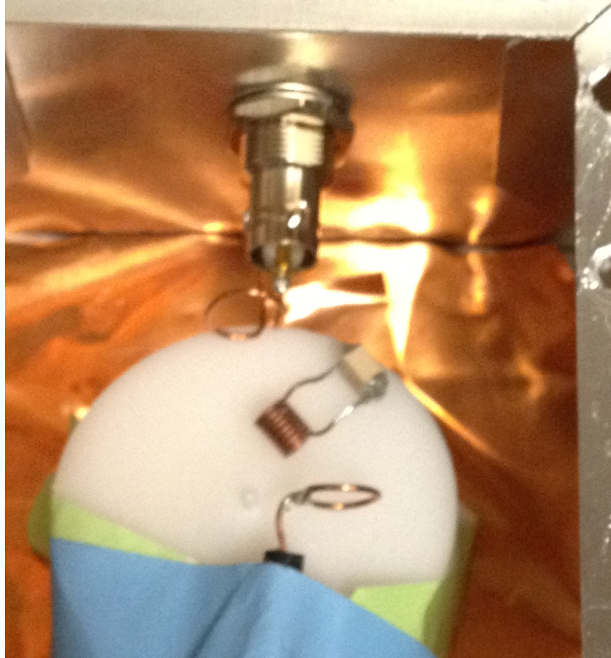
Figure 3.1: Small LC circuit in the "magic box" used to measure resonant frequency.
