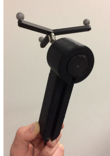
Figure 2-1. tUS transducer in housing
