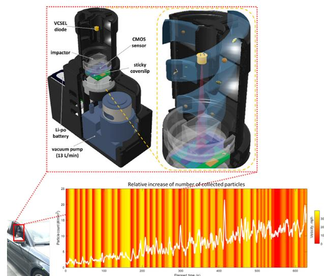
Figure 1. A mobile and cost-effective computational technology to analyze brake and tire wear emissions
