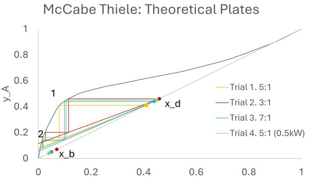
The rectifying line steepens as the reflux ratio increases. All trials resulted in needing two trays to obtain the respective bottoms mole fraction. This results in 25%. column efficiency for all trials.
