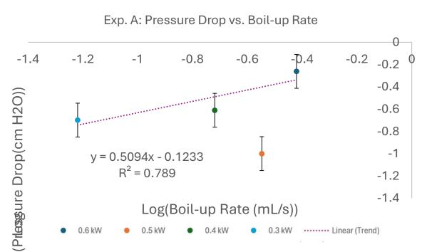
An outlier was seen at 0.5 kW power setting and removed to develop a linear trend on a log-log scale plot. Pressure drop and boil-up rate do not show the expected square relationship.
