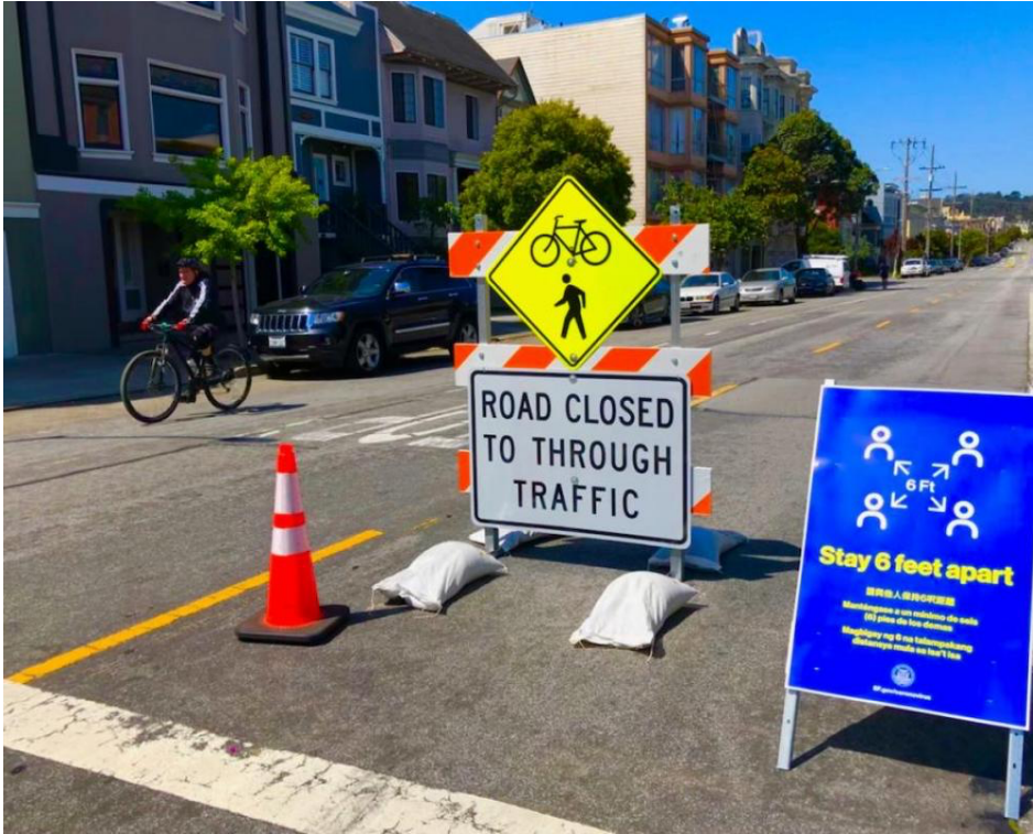
Figure 11: Slow Street signage that doubles as traffic calming, forcing cars entering and exiting to merge lanes before the intersection. Source: SFMTA.
