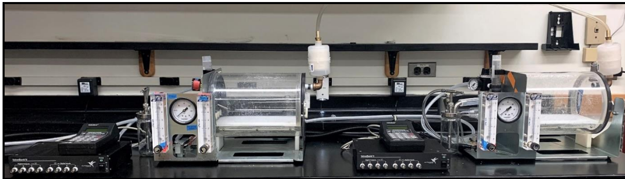
Figure 2. E-cigarette Aerosol Generation Systems. Each chamber housed one C57BL/6 male mouse for the duration of the exposure.
