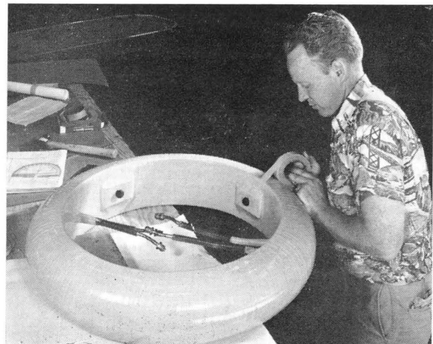
Fig. 13. A Coil of Water-Cooled Square Copper Conductor Being Insulated With High-Strength Polyester Film Tape
