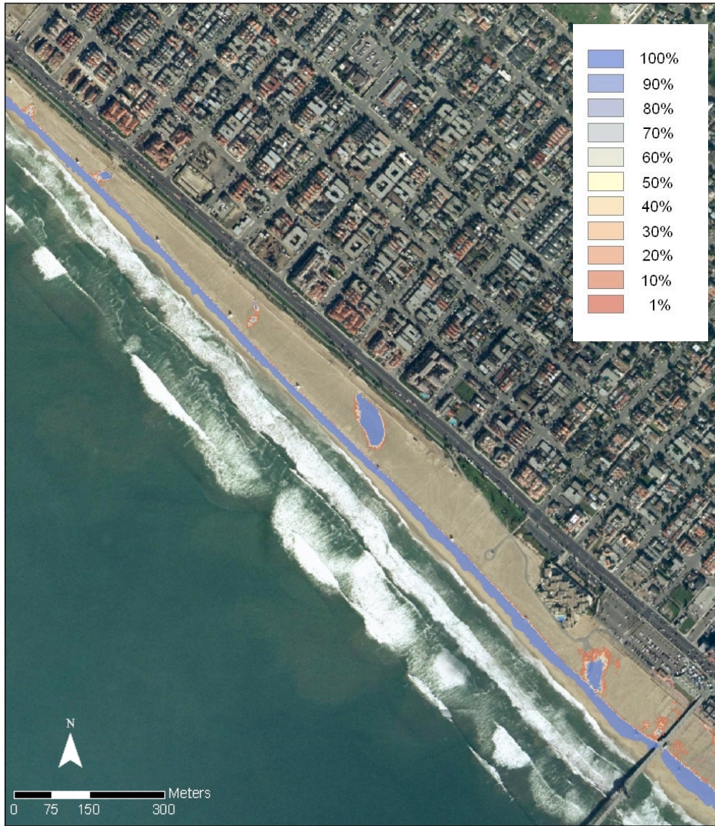
Fig. 2.15: Annual probability of inundation map for Huntington Beach extreme still high water levels with a 140 cm sea-level rise
