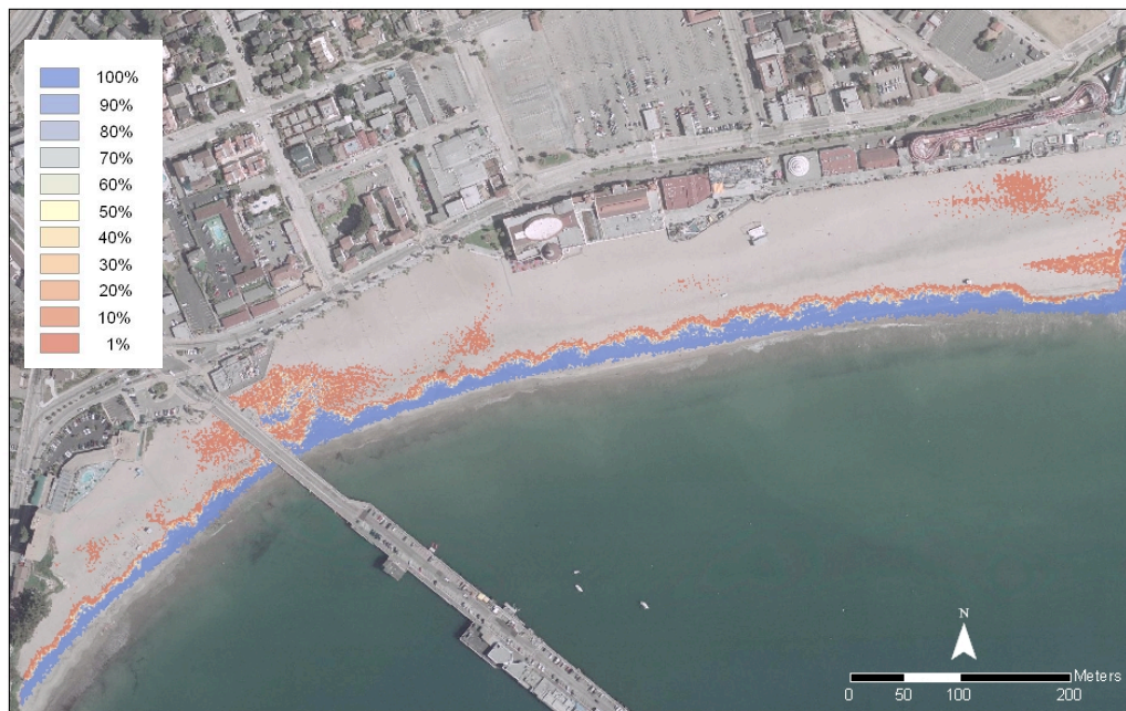
Fig. 2.46: Annual probability of inundation map for Santa Cruz Main Beach extreme still high water levels with an 18 cm sea-level rise
