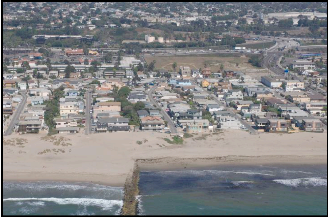
Fig. 2.29: Aerial photo of the characteristic notched planform profile of Ventura Beach due to an extensive alongshore groin field (photo by Kenneth and Gabrielle Adelman)
