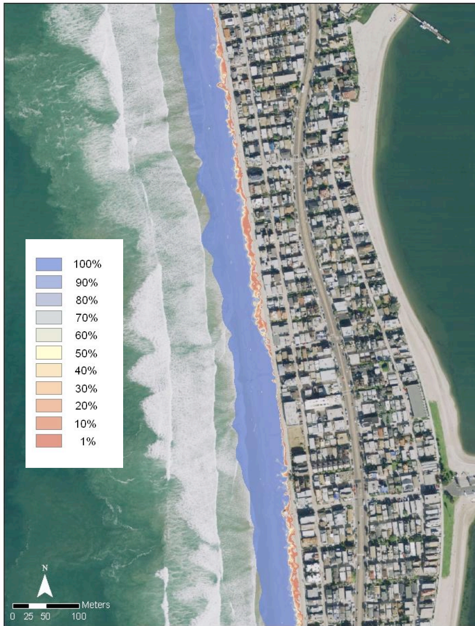
Fig. 2.8: Annual probability of inundation map for Mission Beach extreme still high water levels with 140 cm of sea-level rise
