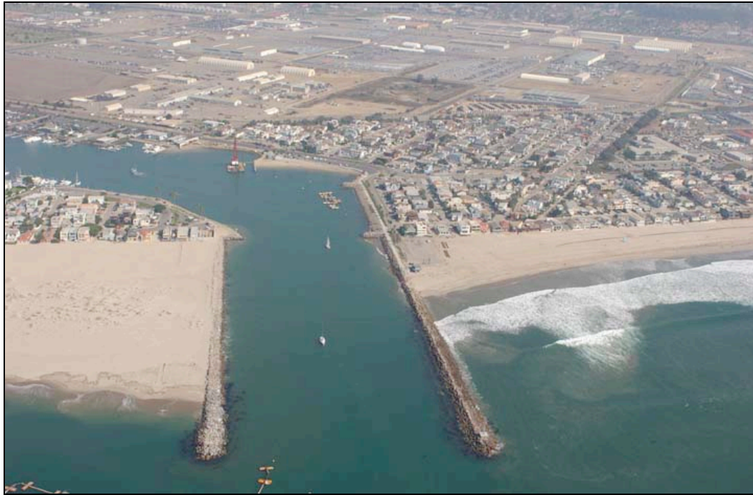
Fig. 1.1: Entrance to the Channel Islands Harbor entrance showing the east and west jetties. The beach has widened updrift of the west jetty and narrowed leeward of the east jetty as a result of the disruption and retainment of littoral drift sediment by the west jetty, resulting in a decreased sediment supply to beaches down drift (photo by Kenneth and Gabrielle Adelman)
