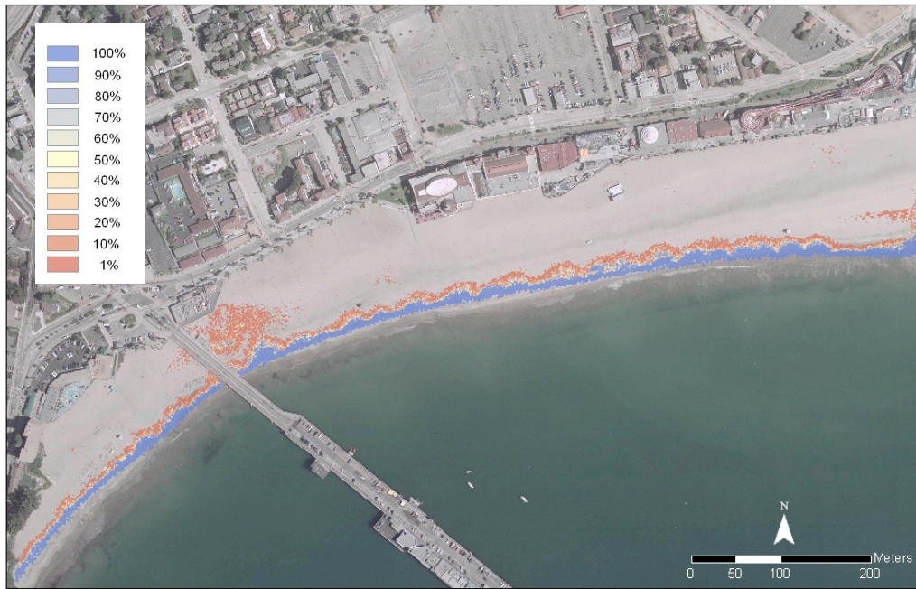
Fig. 2.45: Annual probability of inundation map for Santa Cruz Main Beach extreme still high water levels at current sea-level
