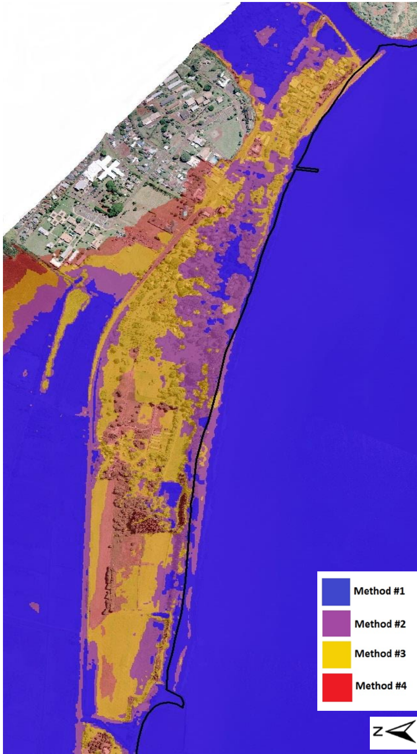
Figure 53 Waimea inundation with 2.0 m of sea-level rise using Methods #1-4
