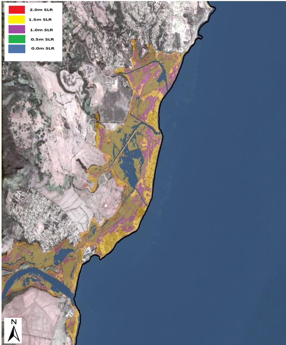
Figure 18 Kapa'a sea-level rise inundation using Method #3
