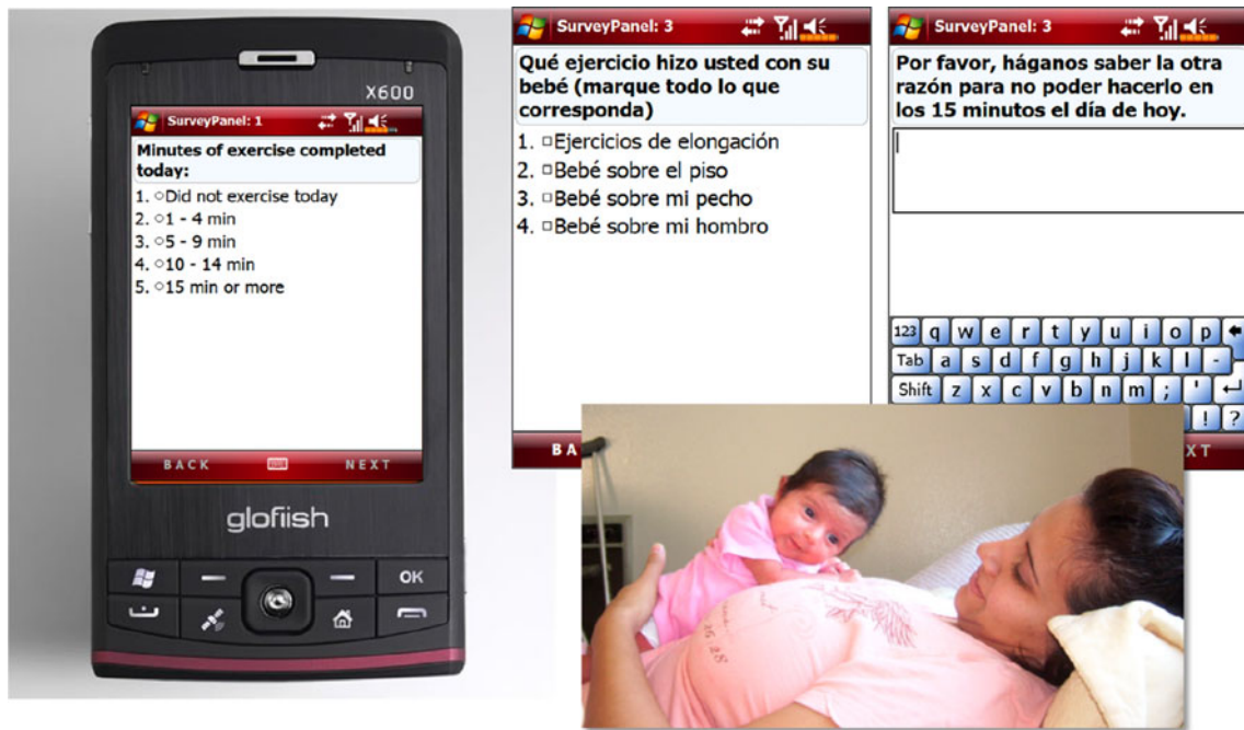
Fig. 5 The FitBaby prototype delivered questions in both English ( left ) and Spanish ( top ) to meet the needs of the target patient population. Mothers could use the phone one-handed while conducting exercises with their infants ( bottom )
