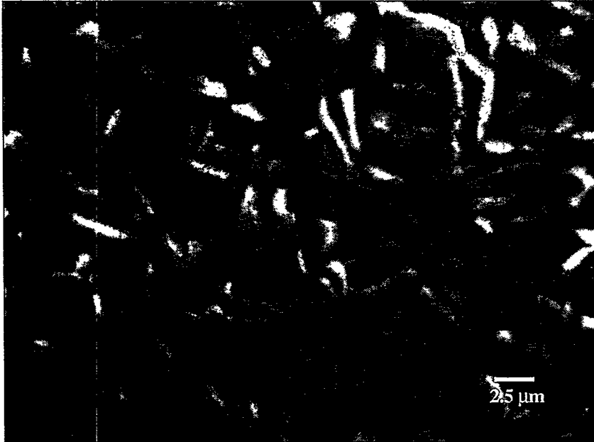
Figure 3.1.5a- SEM picture of \text{Au}_{0.5}\text{Ni}_{0.5}\text{Sn}_4 intermetallic crystals with Pb-Sn solder etched off. Replica samples were made of the individual crystals seen above.
