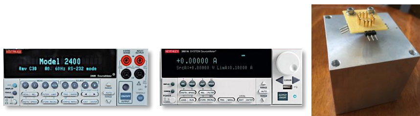
Figure 2.7 | Transport Setup: SMU used for the electrical characterization of the hybrid device. Keithley 2400 for constant current source and measurement of the voltage drop. Keithley 2600 was used to apply bias voltages and measure leakage current in the system. The right panel identifies the metallic leads used to connect the chip carrier to the BNC cables connected to its according SMU
