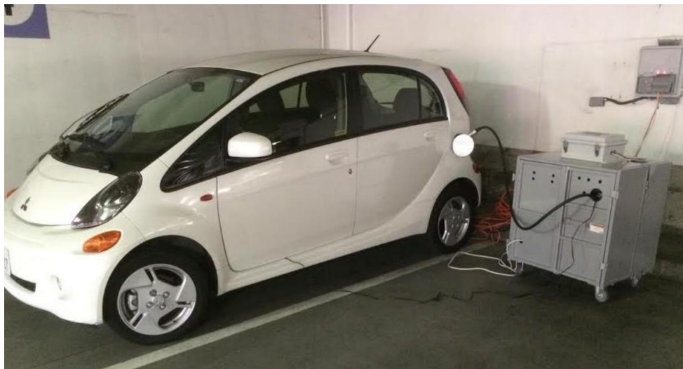
Figure 6-8 Experimental setup of V2H/V2G hybrid system
