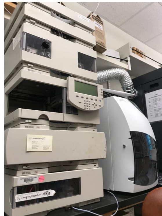
HPLC separates mixtures of compounds based on their physical properties
