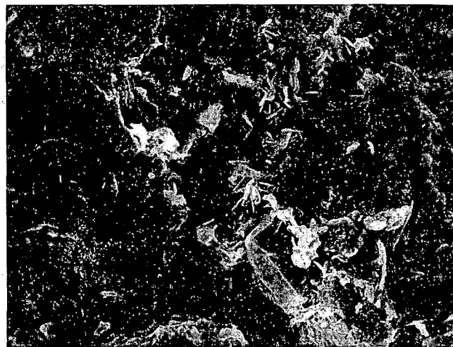
Figure 23. Clay and framework minerals, or mineral overgrowth in a pore space. Sample taken from well M-38, at depths from 1215 to 1372 m; field of view across the SEM photograph is 0.1 mm.
