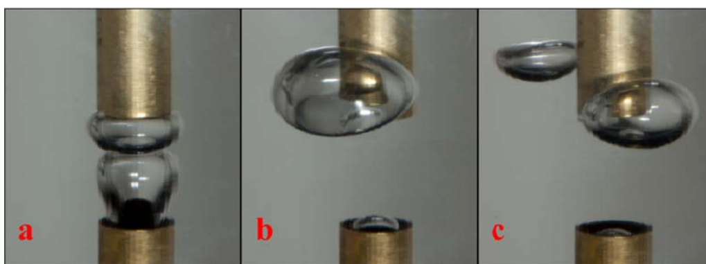
Figure 5.2 Typical behaviors of bubbles in experiments: (a) formation of pairs of bubbles, (b) merged bubble in pure water or \text{NaClO}_4 solutions, (c) separate bubbles in other electrolyte aqueous solution.
