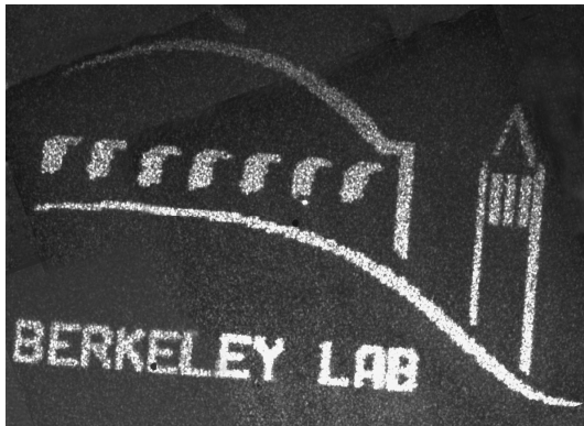
Fig. 4. At-wavelength (13.5 nm) characterization of the fabricated HOE. An imaging detector is used to record the far-field diffraction pattern under low-divergence illumination. Owing to the geometry of the system, it was not possible to record the full extent of the first-order diffraction pattern in a single exposure. The displayed image is a results of stitching several recorded images.
