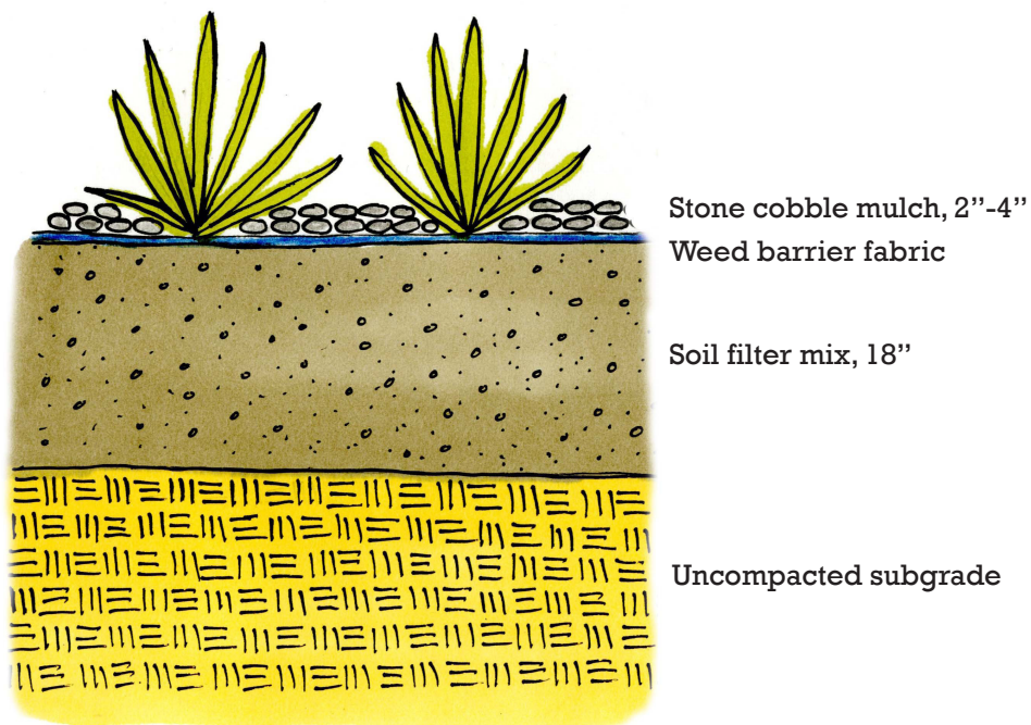
Figure 8. Cross-section of bioretention planter
