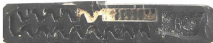
Complete clogging at corner
