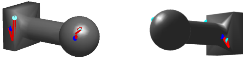
Figure 7.22: The figure shows the path followed by three contact points for object joystick (red line). Each contact point starts from the cyan location and ends in blue.
