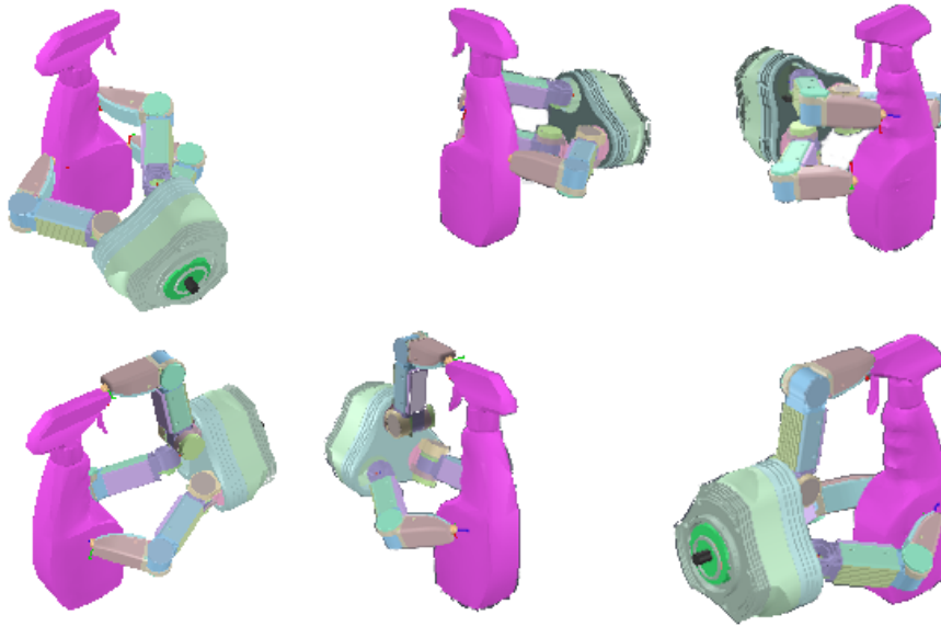
Figure 4.11: Top figures: best grasp determined using the grasp wrench space quality measure. Bottom figures: best grasp determined using the object wrench space quality measure. Each grasp is shown from three different view points to outline the differences.
