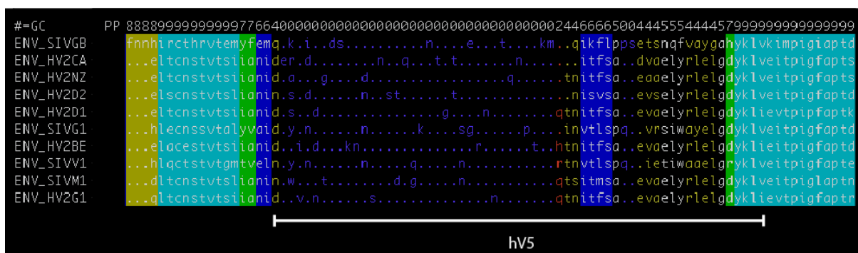
Figure 4.1: A summary alignment of SIV/HIV gp120 proteins produced by constock.pl . Posterior probabilities of alignment columns are shown on the “PP” line (most significant decimal digit) and by ANSI terminal color (white-on-cyan is most reliable, blue-on-black is least). Hypervariable (hV) region 5 [114] corresponds with a low-confidence region.
