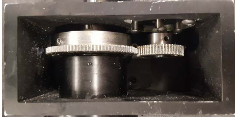
Figure 4. This is a photo taken of the top view of our gear system. The gear on the right connects to the motor's shaft. The larger gear on the left is connected to a bearing housed within the black metal Chassis. This surrounds the rotary joint and controls the speed at which the endoscope rotates.
