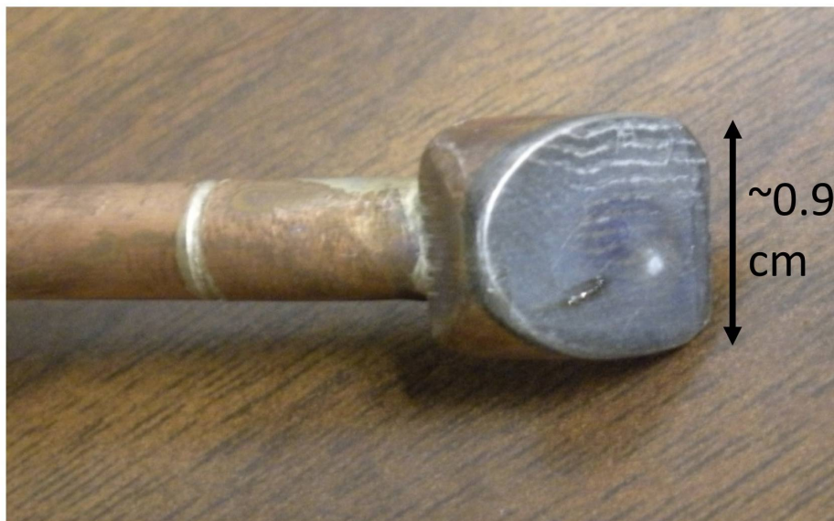
Figure 4.4: A photograph of the target up close, the beam spot is the white colored spot on the target in the photograph, some darkened circles can be seen around it from the heat being dissipated on the target.
