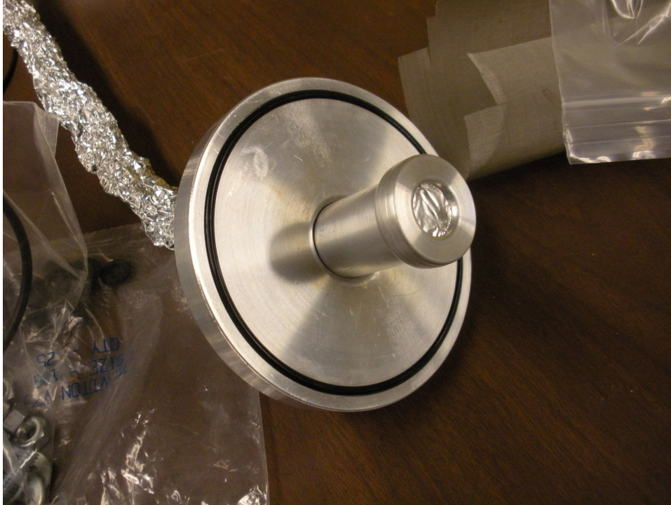
Figure 4.12: A photograph of the charged particle detector with a thin foil in front of it.
