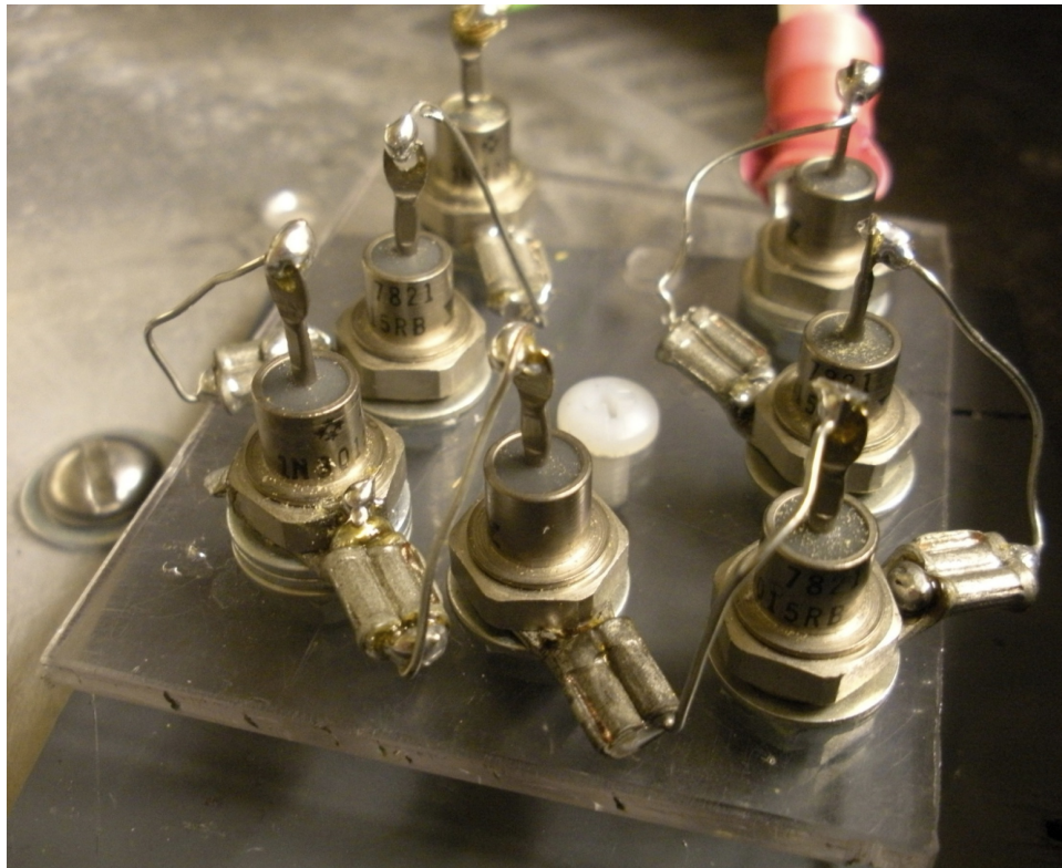
Figure 3.8: Photograph of the Zener diodes. Each diode is capable of providing 200 volts and can dissipate 10 W of power. A 200 M \Omega resistor is connected to ground to ensure there is always current flowing through the diodes.
