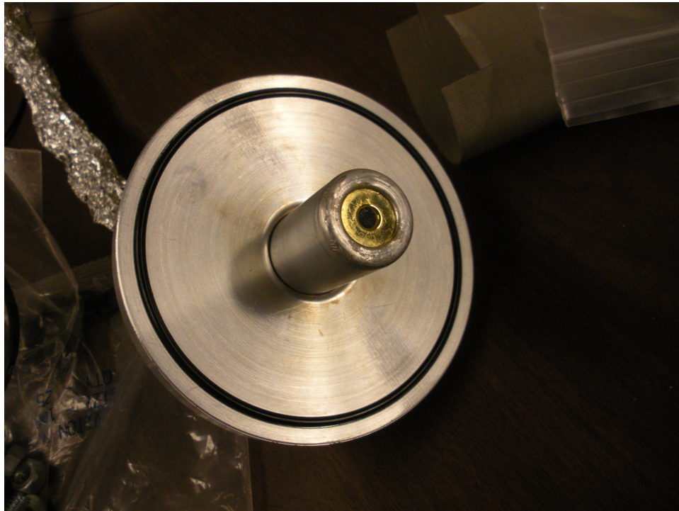
Figure 4.9: A photograph of the charged particle detector.
