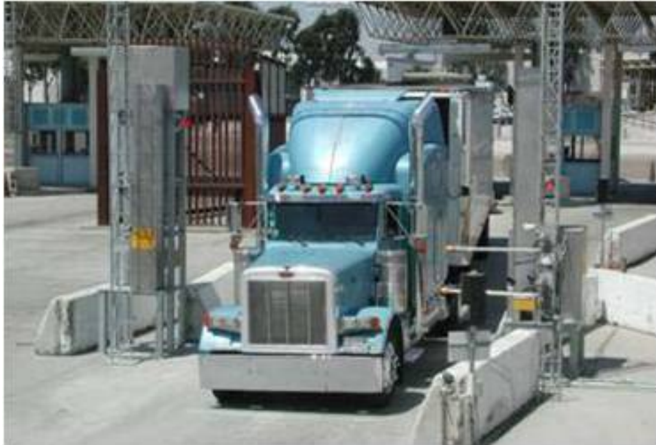
Figure 1.1: Photograph of the Science Applications International Corporation's (SAIC) Vehicle And Cargo Inspection System (VACIS) portal system [4].
