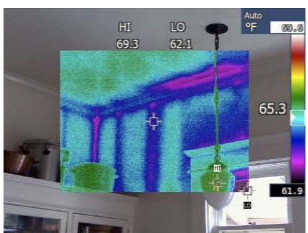
Figure 104 - P7 Post-retrofit problems persist in same location
