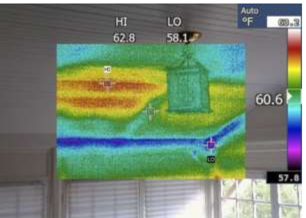
Figure 104 - P7 Post-retrofit problems persist in same location
