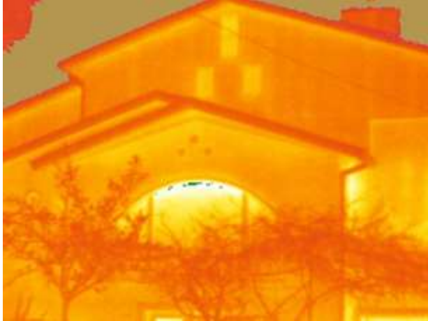
Figure 63 - P4 thermal leakage above honeycomb shade in living room Figure 64 - P4 air leakage around front door
