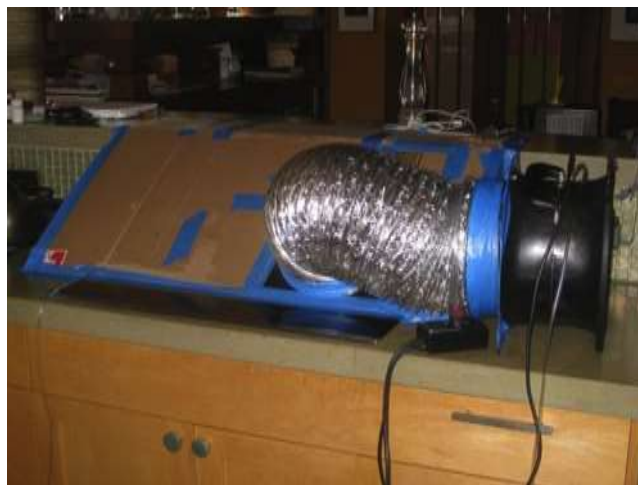
Image 36 - P8 Measuring Airflow of Downdraft Kitchen Exhaust Fan
