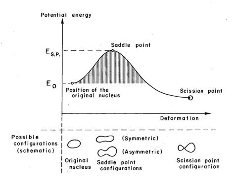
Fig. 1. Spontaneous fission as a barrier penetration problem. The nucleus has to penetrate the shaded area.
