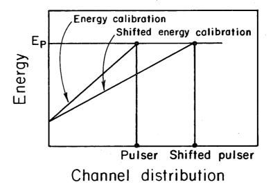
Fig. 26. Correction for the shift in the linear amplification gain as measured with a mercury electronic pulser.
