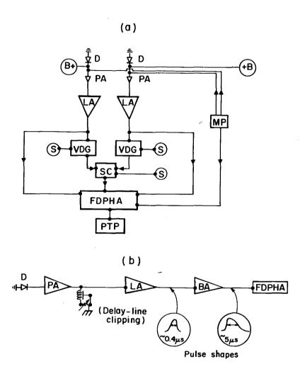
Fig. 25. (a) Electronic system. The components include (D) 1700-Ω-cm phosphorus-diffused silicon detectors, <sup>25</sup> (PA) preamplifiers, (LA) linear amplifiers, (VDG) variable-delay-and-gate units, (S) scalers, (MP) mercury pulser, (B) bias supplies, (FDPHA) four-dimensional pulse-height analyzer, (PTP) paper-tape puncher, and (BA) biased amplifiers.
