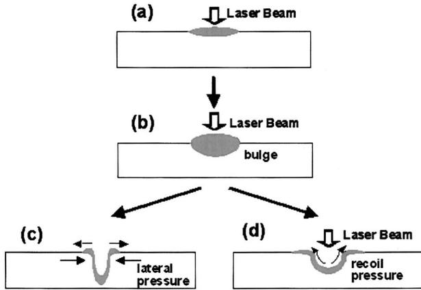
FIG. 1. Schema of proposed mechanism: (a) molten bulge produced by local thermal expansion, (b) flow of bulge caused by surface tension, (c) forming of rim by contraction upon cooling, and (d) forming of rim by recoil pressure.
