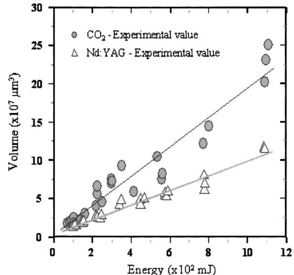
FIG. 5. The changes of pit volume with CO<sub>2</sub> and Nd:YAG laser irradiation.
