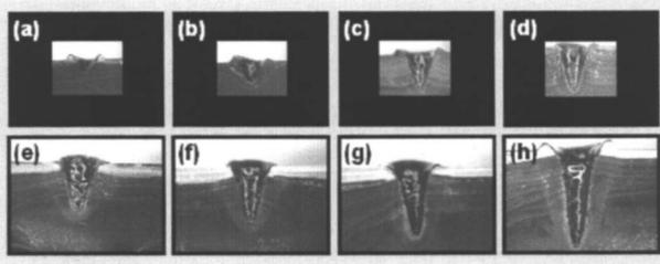
FIG. 2. The cross-sectional view of ABS plastic after CO<sub>2</sub> laser irradiation; (a) 50, (b) 100, (c) 200, (d) 300, (e) 400, (f) 500, (g) 750, and (h) 1000 mJ; 60× magnification.
