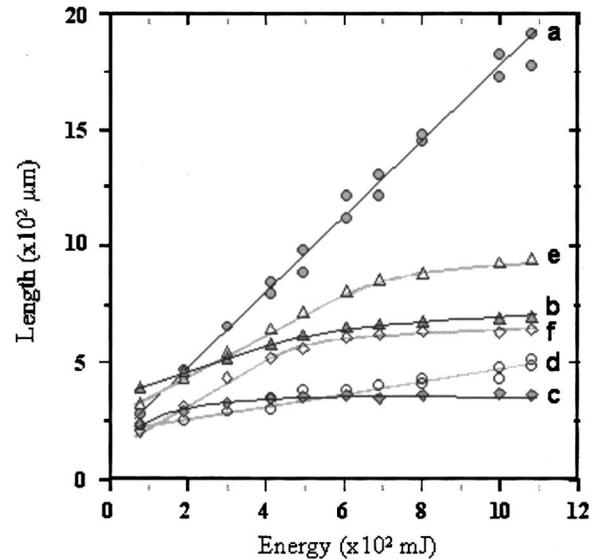
FIG. 4. Changes in depth, width, and FWHM with CO<sub>2</sub> and Nd:YAG laser irradiations; (a) CO<sub>2</sub>—depth, (b) CO<sub>2</sub>—width, (c) CO<sub>2</sub>—FWHM, (d) Nd:YAG—depth, (e) Nd:YAG—width, and (f) Nd:YAG—FWHM.
