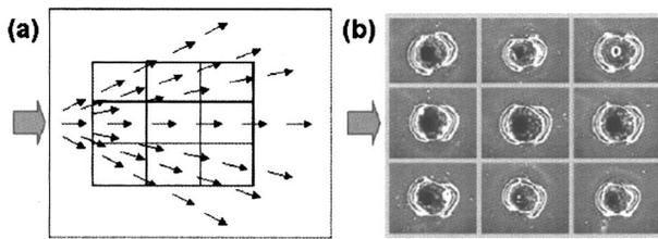
FIG. 6. Photography of laser spot marking on the surface of ABS plastic; (a) traveling course of molten plastic in an injection mold, (b) rim's orientation by laser spot marking corresponding to the injection direction.
