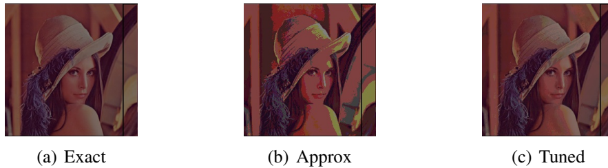
Figure 2.14. Output quality comparison for Blur application running on (a) exact computing, (b) approximate mode ( PSNR = 25dB ), and (c) tuned computing with PSNR = 34dB and 13% run on precise CFPU.
